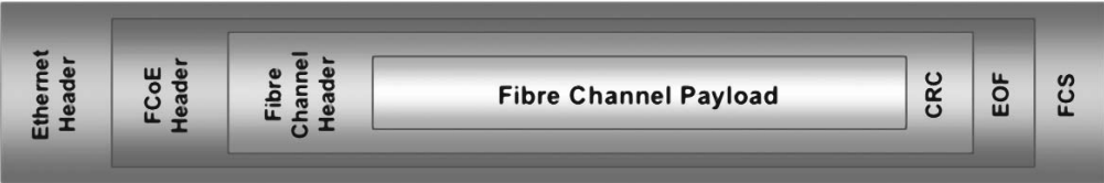
Figure 1 – Ethernet Encapsulated FCoE Frame
