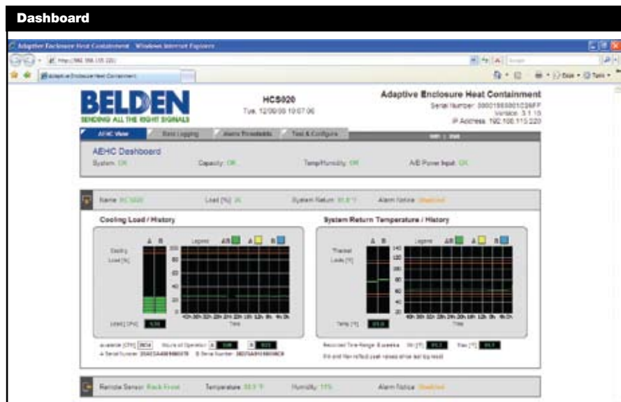
Embedded software allows each AEHC unit to be fully autonomous. The AEHC controllers have their own IP address, enabling network connection. The AEHC then allows for real time monitoring of the heat load, temperature and alarm conditions for each IT enclosure.
