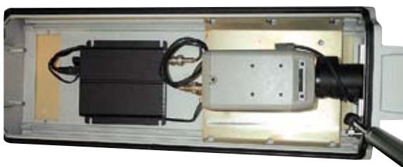
Figure 2. Analog camera with a one-channel video encoder in a camera housing.
